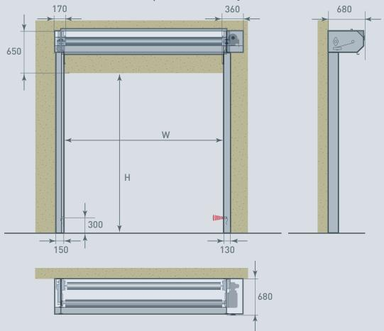
All indicated dimensions are net: the space necessary for mounting and maintenance has to be provided. Remark: drum cover available for doors up to 5900mm wide.
