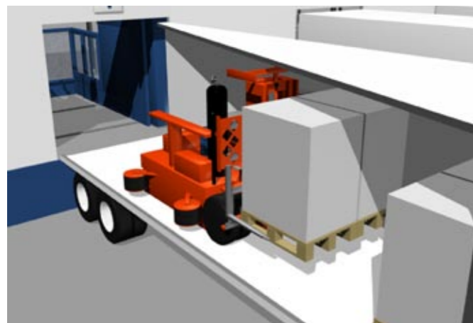
6. ATLS Loading Module enters the truck and deposits the load.
